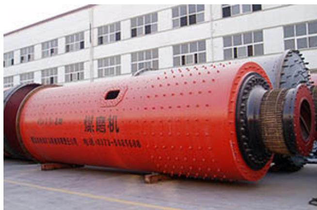
1. It is an efficient tool for grinding coal into fine powder.
